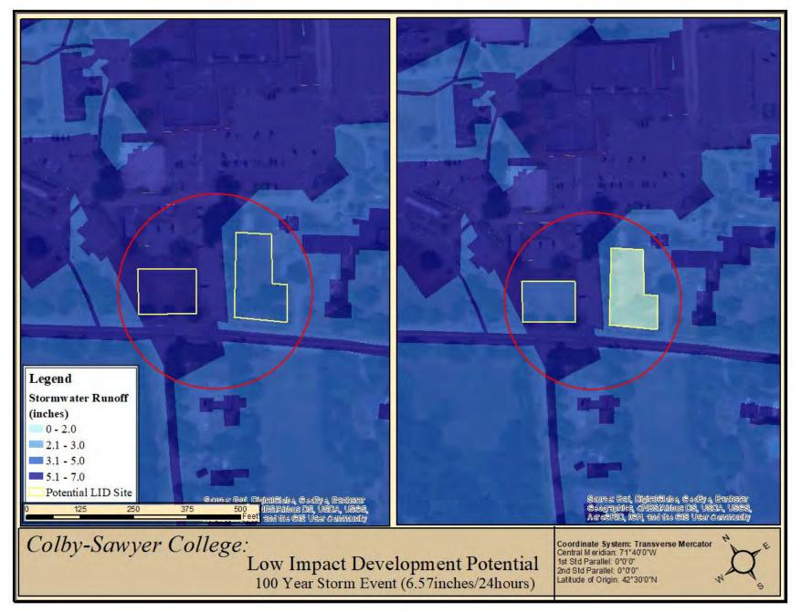
*Figure 27.* Introducing LID sites in the highlighted locations will reduce runoff.
