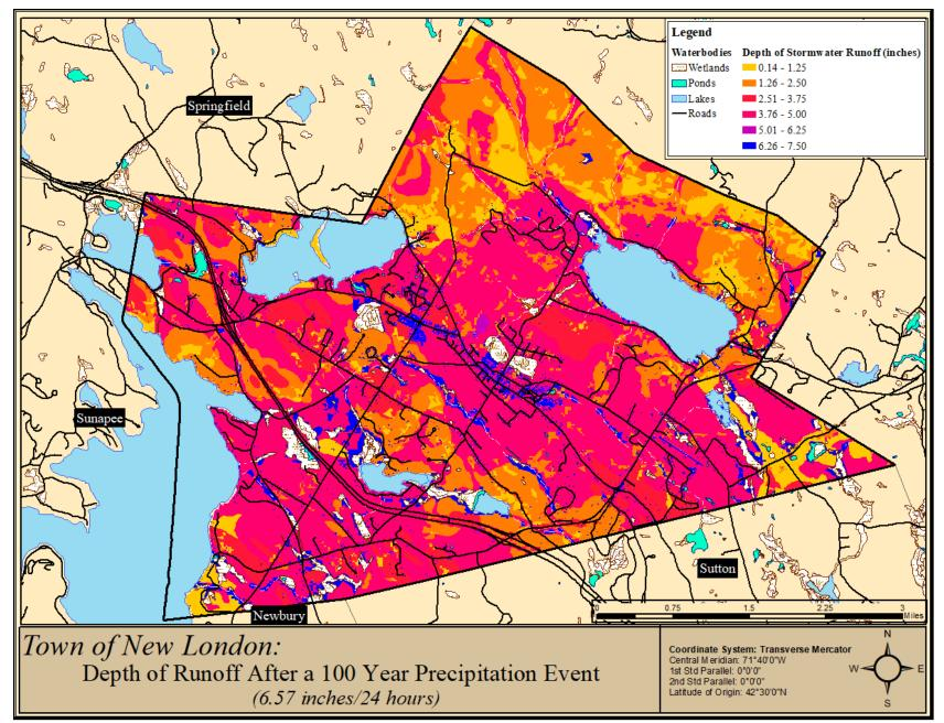
*Figure 22.* Projected depth of stormwater runoff in a 100-year storm event.
